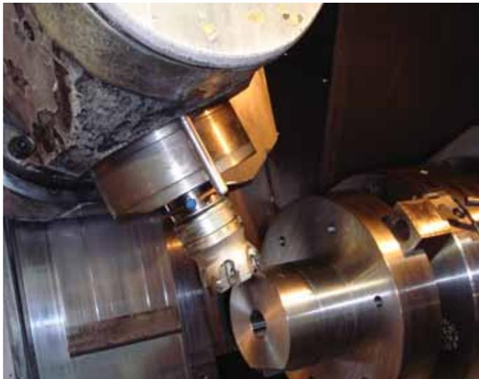
**A natural gas cylinder head nears completion on the subspindle of the Puma MX3000S programmed with GibbsCAM at Paul Precision Machine. The MX3000S can rotate its coordinate system along the B axis to act as a vertical mill. The final operation of milling 120° flats is done with a 3" (76-mm) Mitsubishi face mill.**
