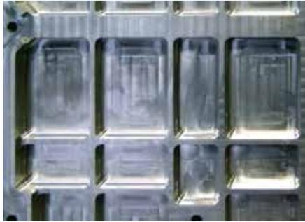
**GibbsCAM VoluMill optimizes tool paths for fast material removal while compensating for changes in cutting direction. Here is a close-up of a 9-by-11-inch instrumentation cover. The toolpath used a  $\frac{5}{16}$ -inch end mill on pockets measuring 0.750 to 1.250 inches wide.**
