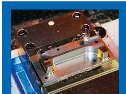
**In a recent field application, PTD Manufacturing used UHPT technology to cut out this part, more than doubling machining efficiencies over its previous solution and illustrating the large quantities of metal that can be easily and quickly removed.**
