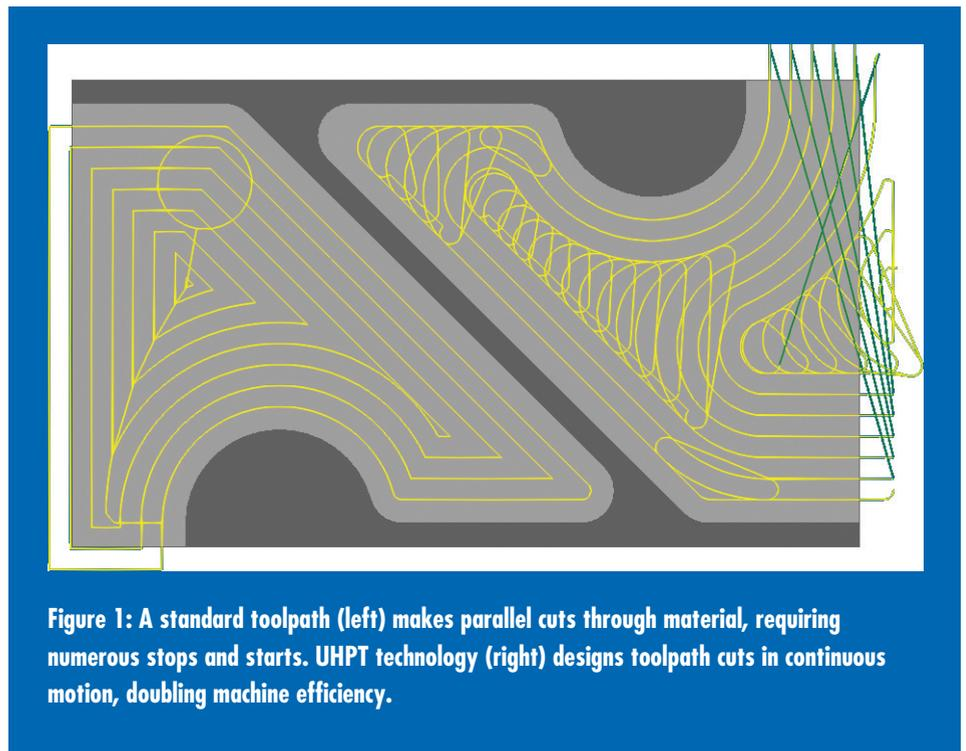
**Figure 1: A standard toolpath (left) makes parallel cuts through material, requiring numerous stops and starts. UHPT technology (right) designs toolpath cuts in continuous motion, doubling machine efficiency.**
