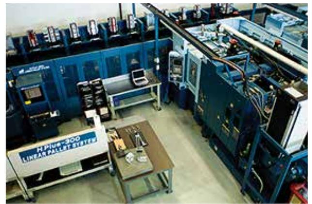
**Redline’s success in unattended machining (seen here) comes from predictable programming, tight process control and good technology.**
