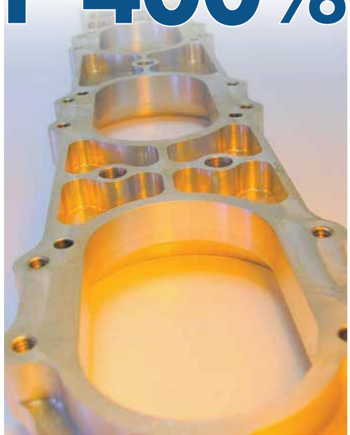
*VoluMill technology makes maximum use of the tooling available in the shop of Quelch Engineering to extend machine tool life and greatly reduce cycle times on complex jobs such as this.*
