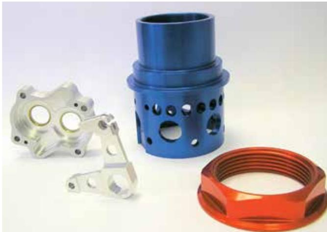
*The CAM software enables the programmer at Quelch Engineering to rough as deep as possible and make use of the full length of the tool. It then automatically re-roughs the large steps produced, ready for part finishing.*
