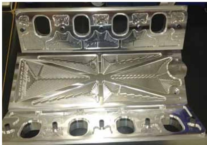
**Manifold valley and flanges machined from billet show the pattern VoluMill creates when it generates the most efficient toolpath motion for running at maximum rpm and feed rate while machining the 1/2" (12.7-mm) deep pockets in a single pass. Switzer leaves the machined finish to demonstrate part quality and beauty.**
