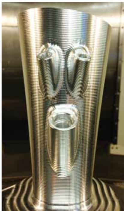
**Completed runner is programmed with GibbsCAM five-axis software and machined from aluminum billet in four-axis with a wall thickness of 0.090" (2.3-mm) to replace sheetmetal fabrication. Built-in bungs eliminate the previous welding and manual machining required for sheetmetal runners.**
