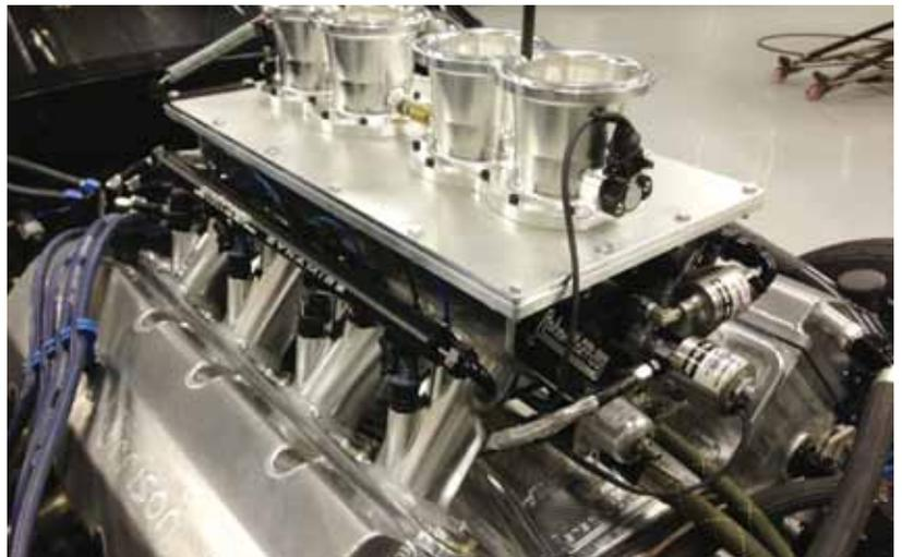
***New Switzer Dynamics intake manifold made for Reher-Morrison Racing Engines qualified with a first place at its debut at Bristol in April 2013. Previously fabricated from sheetmetal, it's now made with components machined from aluminum billet and programmed with GibbsCAM.***
