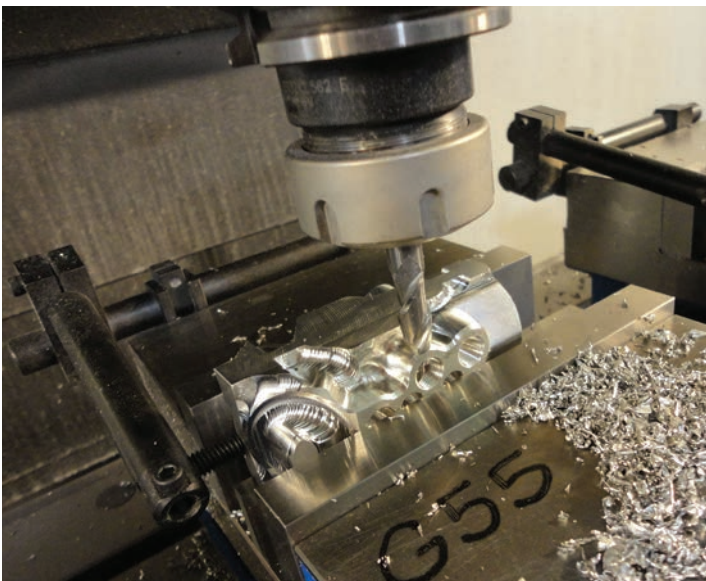
One in a row of five magnesium Y blocks mounted on the Kalitta Motorsports Haas VF-4 CNC, shown here between operations.
